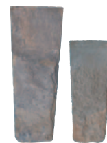
Swept valley slip slates
